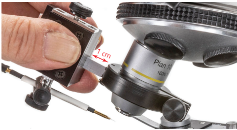
Fig. 7—Mounting the Filament Adjustment Assembly
