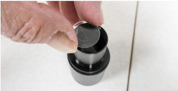
Fig. 30—Insert the reticle with the text on the bottom side of the reticle.
